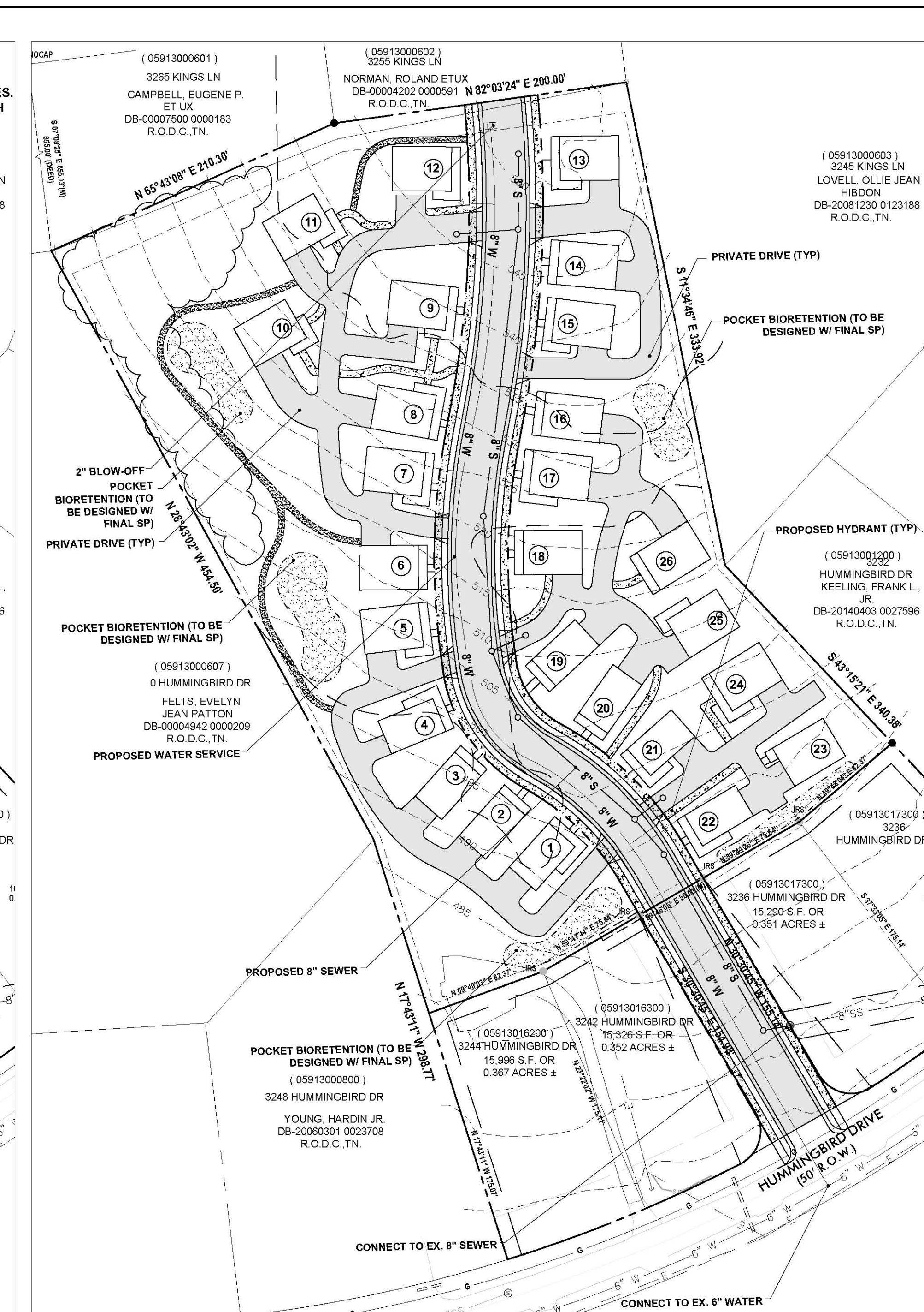
Proposed Utility & Grading Plan (1"=60')
