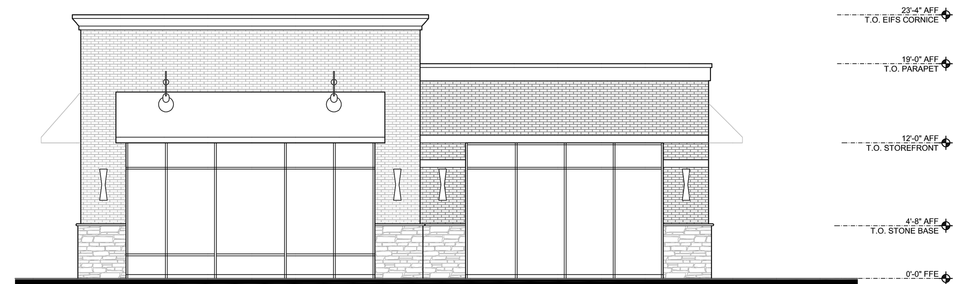
3 SIDE (EAST) ELEVATION 3/16" = 1'-0"
