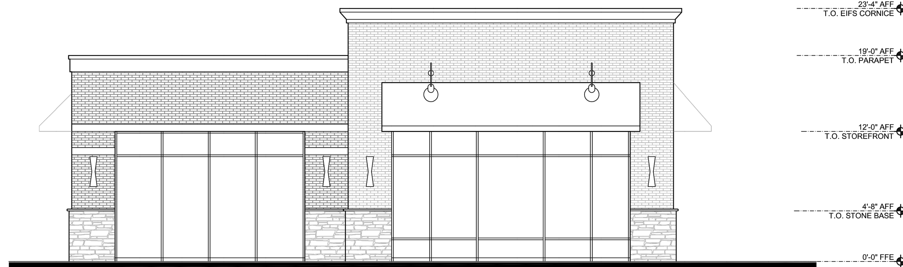
2 SIDE (WEST) ELEVATION 3/16" = 1'-0"
