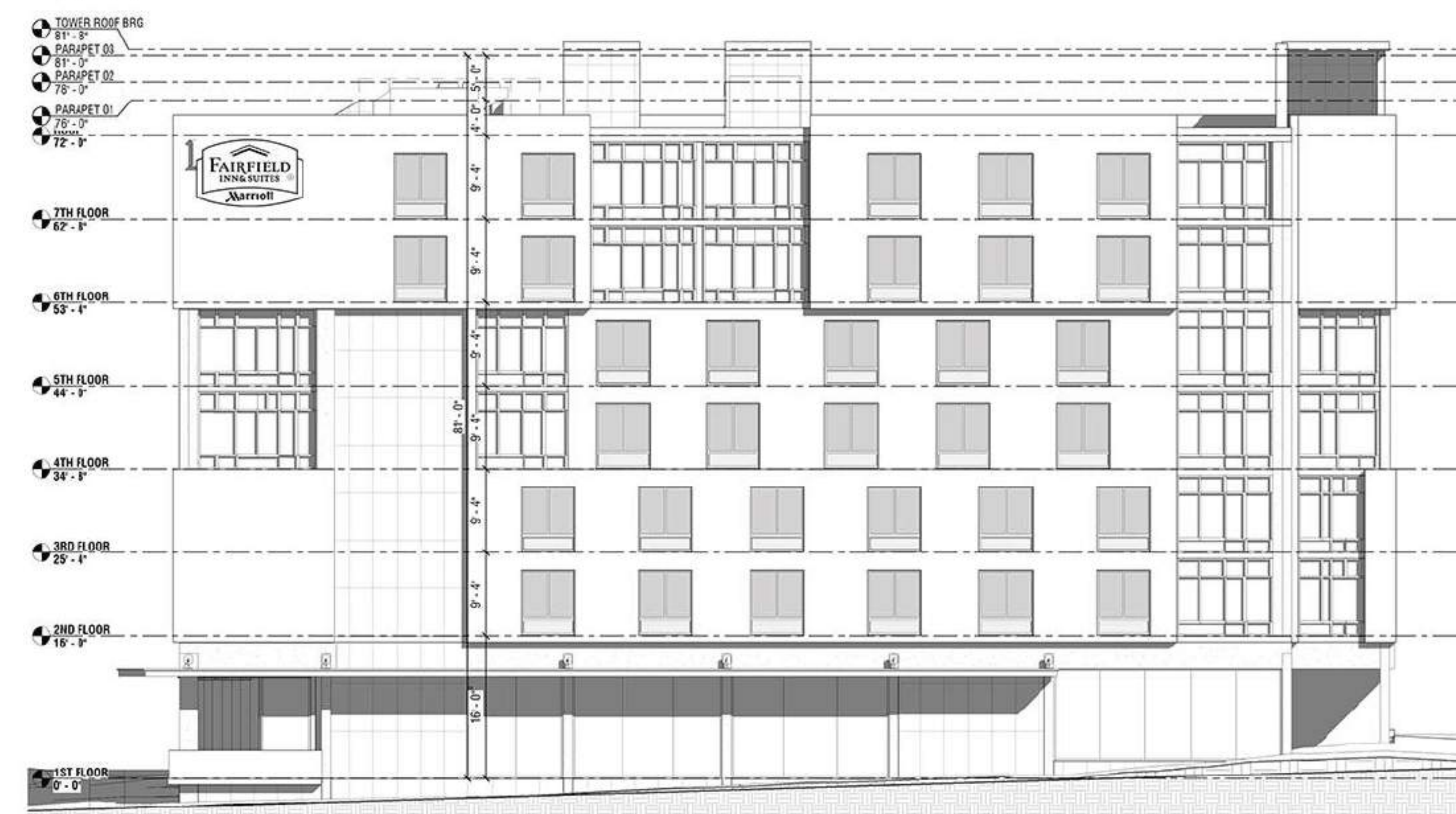
① EXTERIOR ELEVATION: RIGHT 3/32" = 1'-0"
