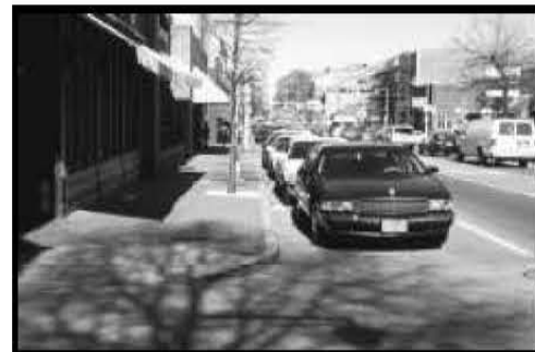
On-street, parallel parking can serve as a buffer between the pedestrian and the automobile, as well as a traffic calming measure.
