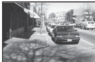
On-street, parallel parking can serve as a buffer between the pedestrian and the automobile, as well as a traffic calming measure.
