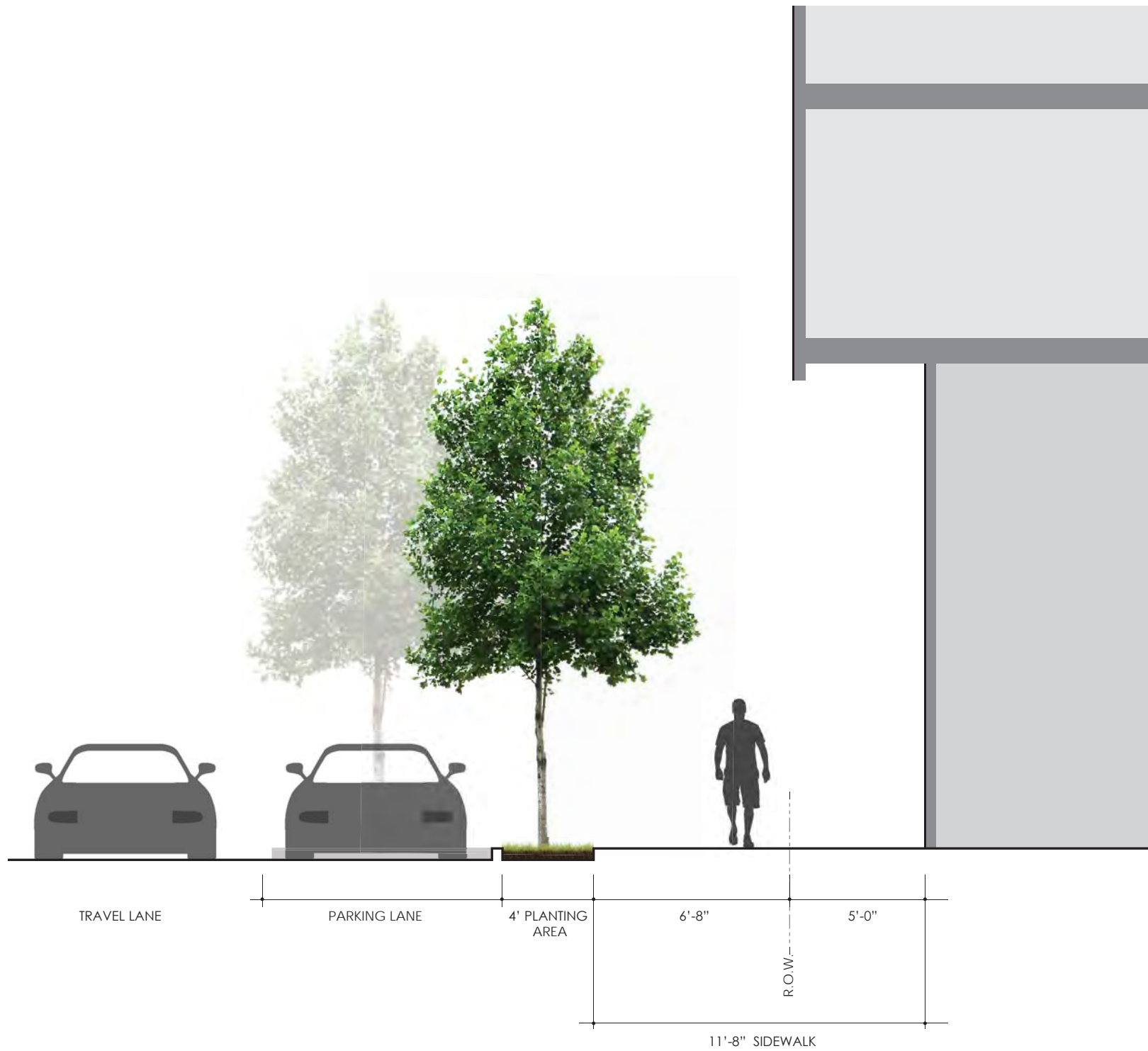
SECTION AT VANDERBILT PLACE SIDEWALK
