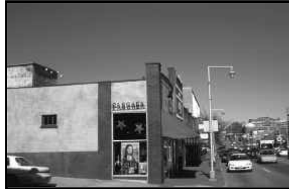
Flat roofs with parapet walls are the dominant form in the Village's commercial core.
